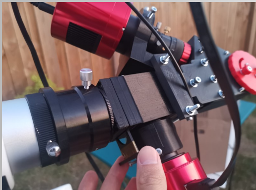
Fig.5: The polarimeter is placed in front of the spectro guide cube. Closer to the slot would have been better to limit the optical defects of the flexible lenses of the glasses but I wanted to make it as simple as possible in terms of assembly.
